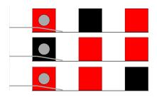
\* robot.sense\_color() returns the color of the box in front of the sensor, or no color('') if no box detected.
