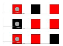
\* robot.sense\_color() returns the color of the box in front of the sensor, or no color('') if no box detected.
