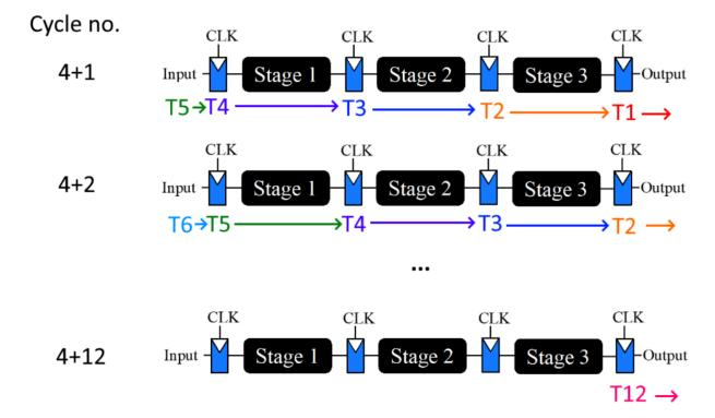
In total, it will take 4 + 12 = 16 cycles till all tokens have been outputted. Given the clock period of 4 ns, this means a time of 16 cycles \* 4 ns per cycle = 64 ns.
