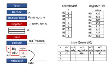
Pipeline cycle-by-cycle diagram format:
