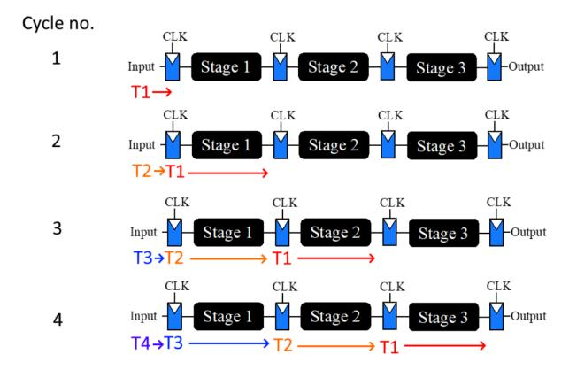
In this diagram, the tokens are labeled T1, T2, and so on. Note that because of the register sitting in front of stage 1, the first token cannot actually start Stage 1 until one clock cycle has passed.
