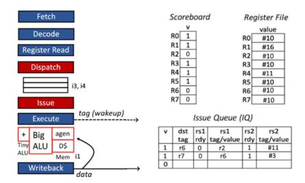
Pipeline cycle-by-cycle diagram format:
