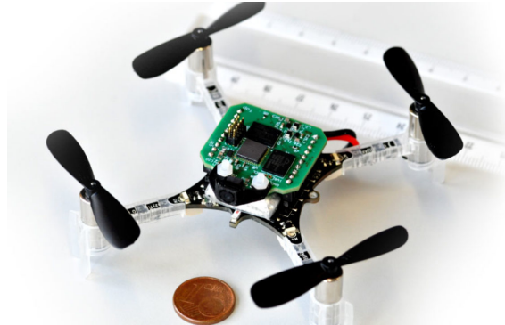
Self-flying nano drone 94 milli-watts
