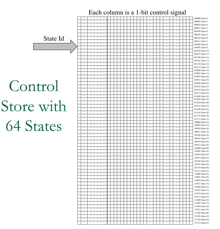
Each entry in the control store is a microinstruction corresponding to the FSM state
