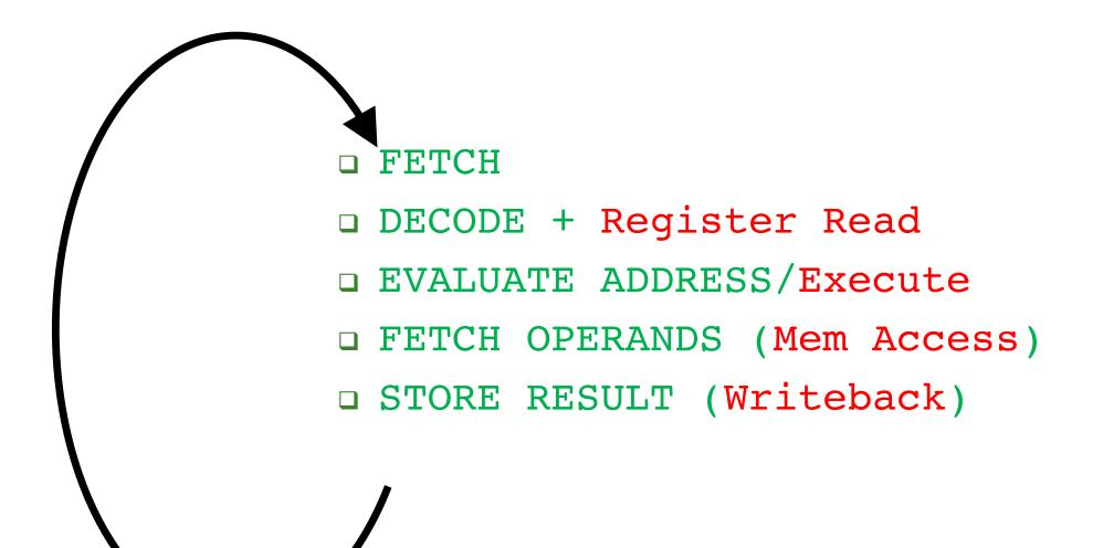
Instruction Processing "Cycle" vs. Machine Clock Cycle
