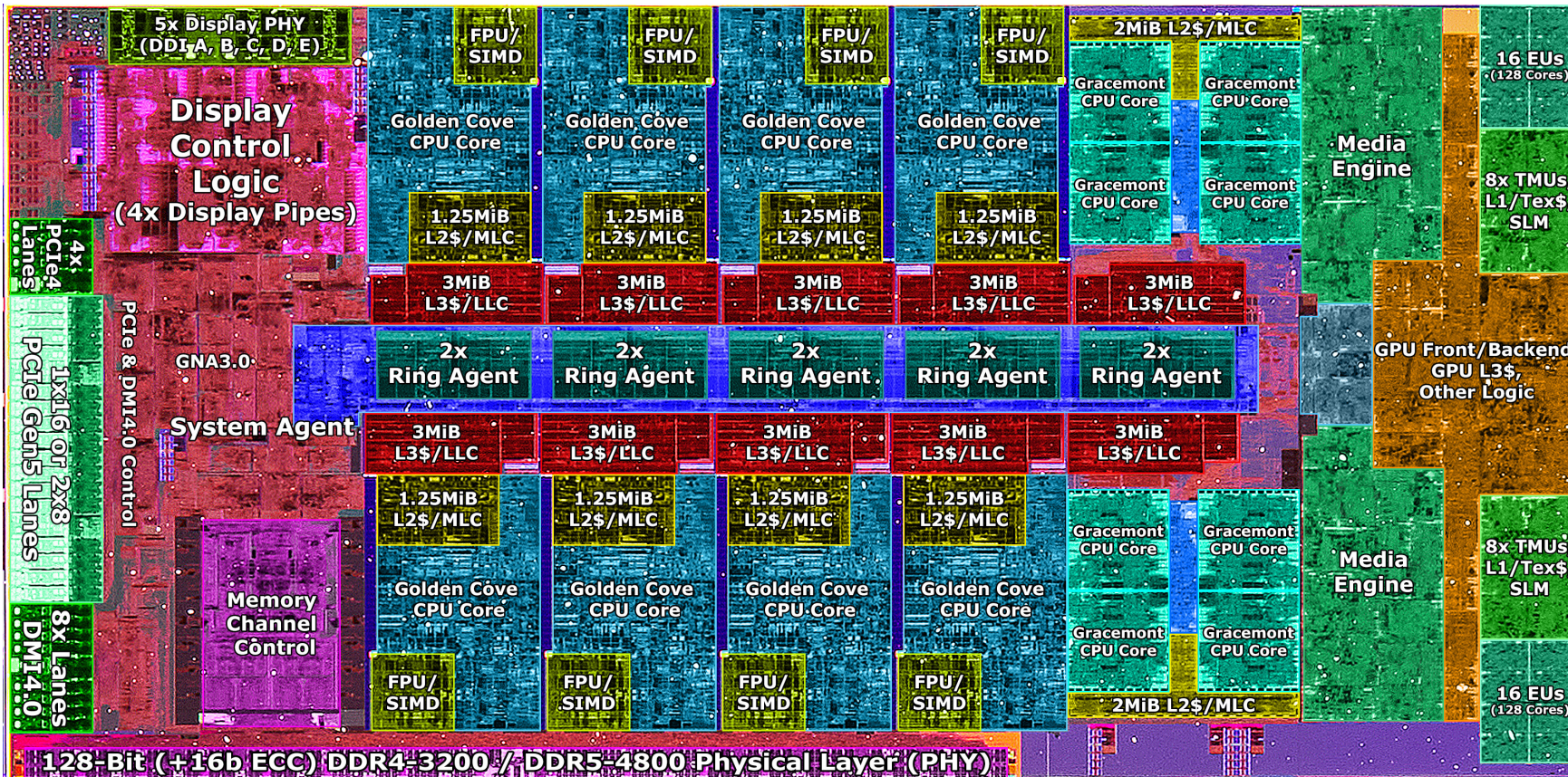
10nm ESF=Intel 7 Alder Lake die shot (~209mm 2 ) from Intel: https://www.intel.com/content/www/us/en/newsroom/news/12th-gen-core-processors.html Die shot interpretation by Locuza, October 2021
