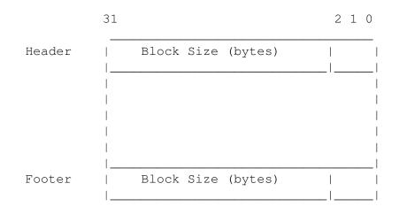
Each memory block, either allocated or free, has a size that is a multiple of eight bytes. Thus, only the 29 higher order bits in the header and footer are needed to record block size, which includes the header and footer. The usage of the remaining 3 lower order bits is as follows:
