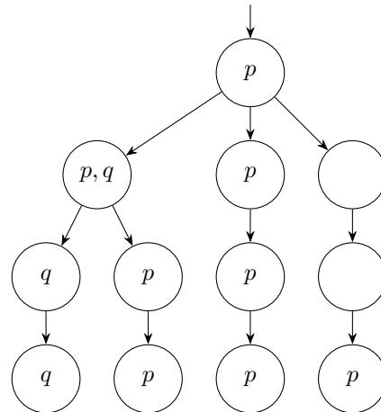
Suppose each path through the tree continues, below the lowest level drawn, without branching or changing how propositions are labelled. Draw a transition system that has this computation tree.
