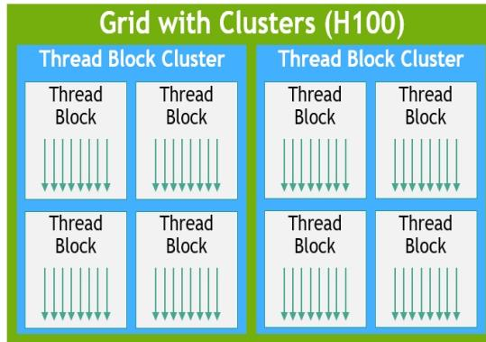
A Grid is composed of Thread Blocks in the legacy CUDA programming model as in A100, shown in the left half of the above diagram. The Hopper architecture adds an optional Cluster hierarchy, shown in the right half of the diagram.
