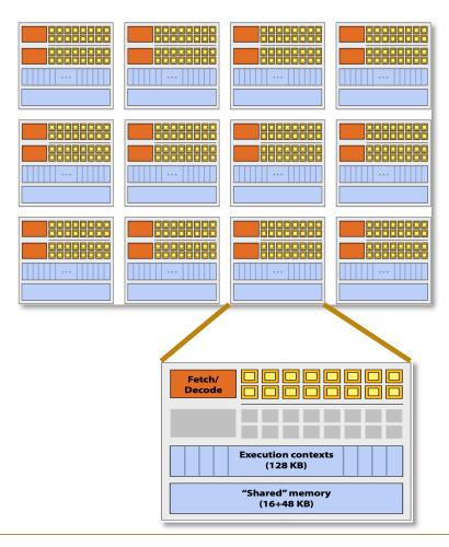
A scalable array of complex "cores" called Streaming Multiprocessors (SM)
