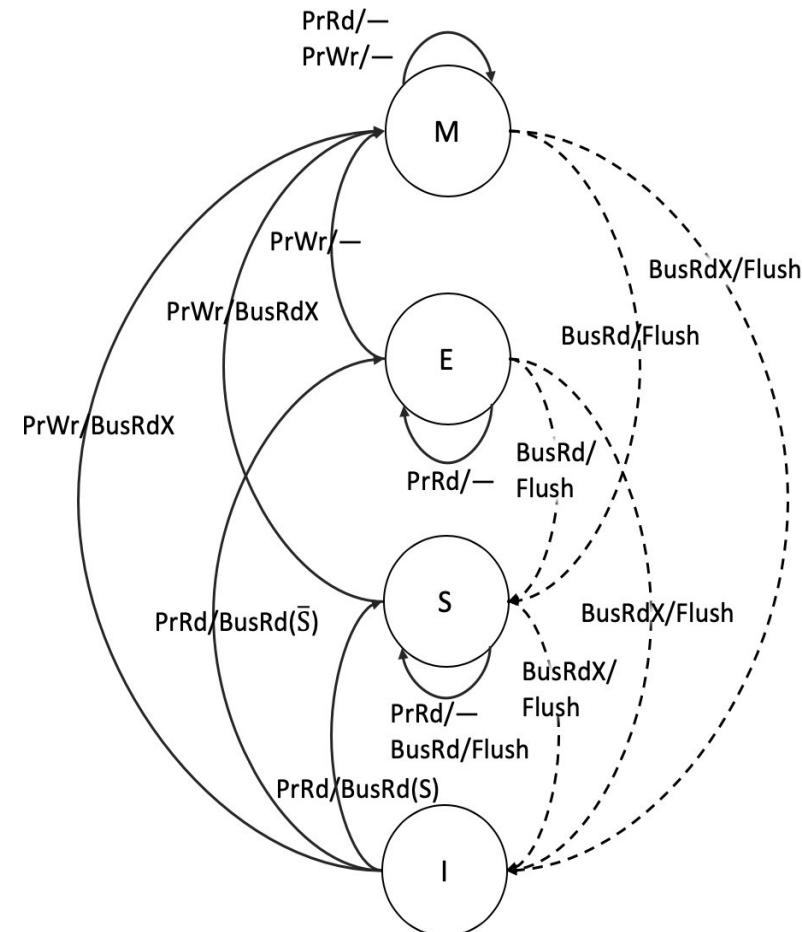
A / B: if action A is observed by cache controller, action B is taken
