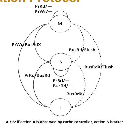
A / B: if action A is observed by cache controller, action B is taken
