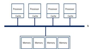
➤ A **shared memory multiprocessor (SMMP)** is one that offers the programmer a single physical address space across all processors – which is nearly always the case for multicore chips – although a more accurate term would have been shared-address multiprocessor.
