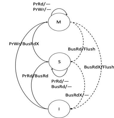
A / B: if action A is observed by cache controller, action B is taken
