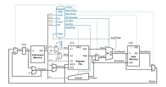
$t_{pcq\_pc} = 35 \text{ ps}, t_{mem} = 180 \text{ ps}, t_{dec} = 70 \text{ ps}, t_{mux} = 25 \text{ ps}, t_{RFread} = 110 \text{ ps}, t_{ALU} = 128 \text{ ps}, and t_{RFsetup} = 66 \text{ ps}$
