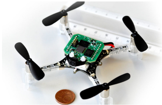
Self-flying nano drone 94 milli-watts
