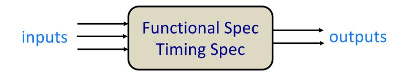
Functional specification: What is the circuit supposed to do? What is the output for a given combination of input values?
