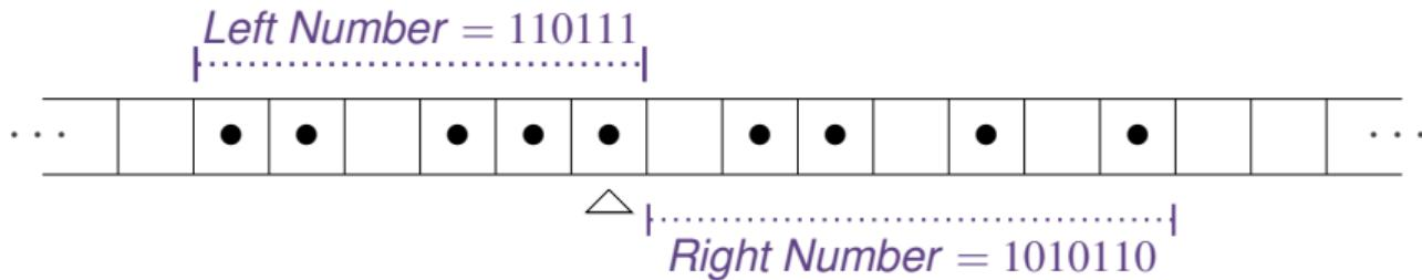
Tape portions to the left and right of the r/w head can be seen as a binary number, with least significant bit nearest to head.
