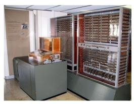
2600 relays 5-10 Hz 22 bit words 4 kW
